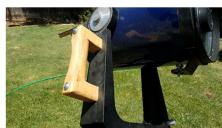
The next item I made is extremely practical for carrying and mounting my Meade 8"SCT. I've needed a big comfortable handle for the longest time. It is made for a chunk of 2x4 and bolted right through the fork. What a difference this has made. Sometimes, very simple things can bring great joy.
